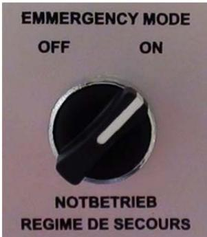
4. Turn the "EMERGENCY MODE" switch to position "ON" (*only for UNIVERSAL PRO & PRO-G control unit*).
