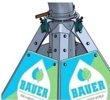
Two momentary-contact limit switches are mounted on the *pivot*, which can be fixed at the desired position for setting the sector. The limit switches are actuated by a switching bracket mounted on the pivot infeed elbow.
