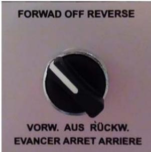
5. Turn the "FORWARD - OFF - REVERSE" switch to "FORWARD" or to "REVERSE" in order to start the system in the desired direction (*only for UNIVERSAL PRO & PRO-G*).
