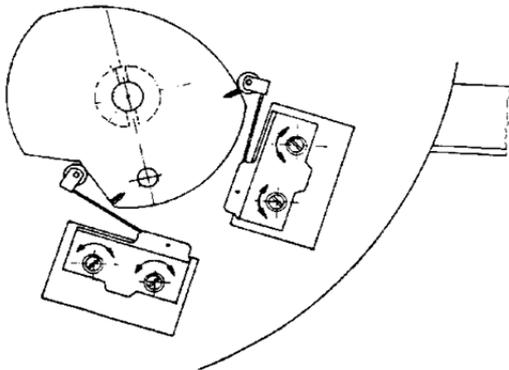
b) To set the control switch, rotate the switching cam until the roller rests in the notch "A". Adjust the switch in the boltholes towards the switching cam until the control switch (micro switch) actuates (clicks). Thereby the bracket of the switch lies near the switch housing.
