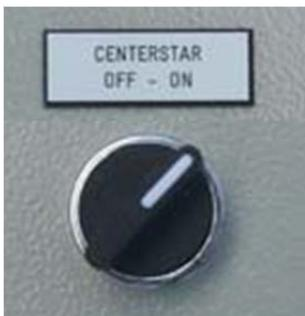
4. Turn "CENTERSTAR ON - OFF" switch to "ON".
