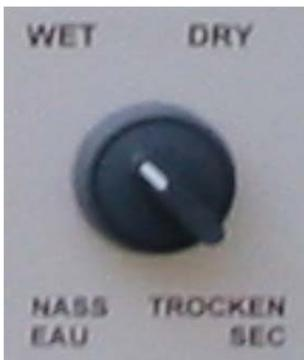
4. Turn the "WET – DRY" switch to the requested position according to the required operating mode.
