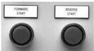
5. Press the green "FORWARD START" or "REVERSE START" pushbutton and hold it depressed until the electric switch audibly actuates and the towers start moving.
