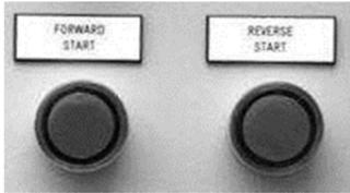
3. Set proper running direction. Select that direction that brings the outermost system end into radial alignment.
