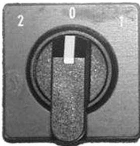
6. Actuate the tower alignment switches in order to align the towers with the pivot centre (sight over the drive motors).
