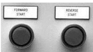
5. Press the green "FORWARD START" or "REVERSE START " button and hold it depressed until the towers start moving.
