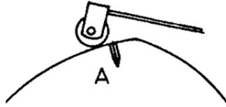
3. Turn back the operating cam by half of the nut or wrench rotations counted under point 2 above - the roller is positioned exactly in the middle between switching and reversing point of the control switch.
