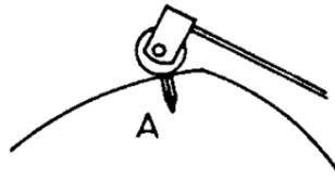
2. Rotate the operating cam clockwise to the reversing point of the control switch, counting the number of rotations of the hex. nut or wrench turns.
